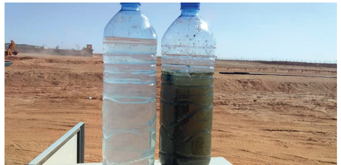
Clarity of the System O)) effluent compared to the affluent
