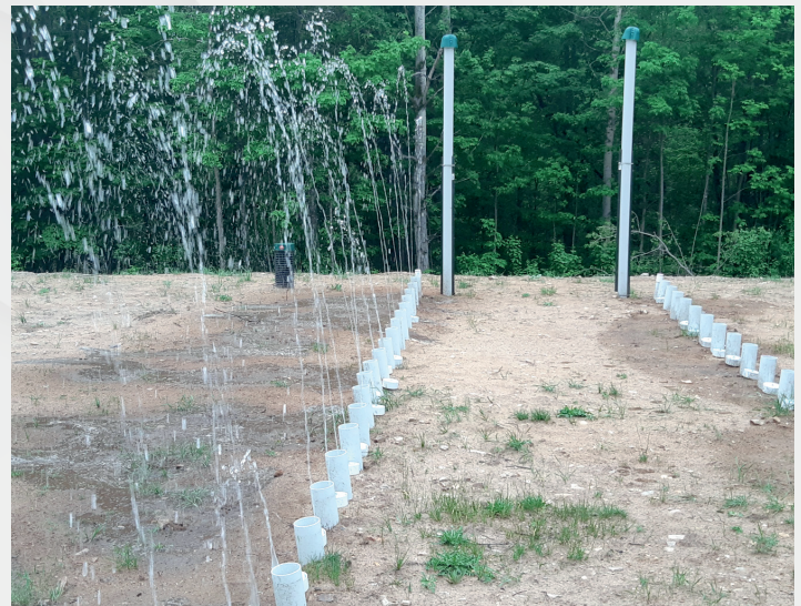
Calibrating the low-pressure headers
